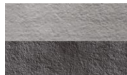
CSP-3 Light Abrasive Blast
